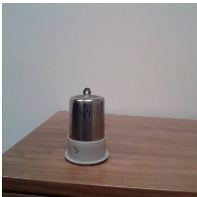
Fig.(2b) : Closed-Cup tube for SSNTD technique
